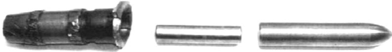
Figure 2.2.26 — Elements of a bullet with a tandem core of a cartridge (ammunition) 12,7×55 (SC-130 VPS) after defeat of the purpose
